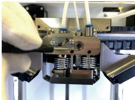
3. Turn off the Composer and tighten the bolt. While tightening servo will rotate to its max angle and stop so you can tighten it
