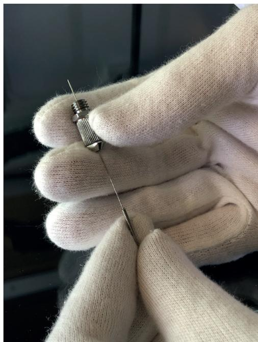
**NOTICE:** Fiber guiding bushing consists of two parts. If you face any problems while cleaning the channel, you can disassemble it and clean the parts separately
