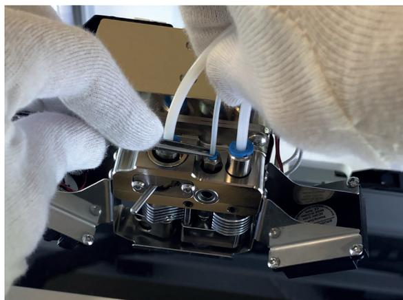
2. Remove the excess fibers from the tube
