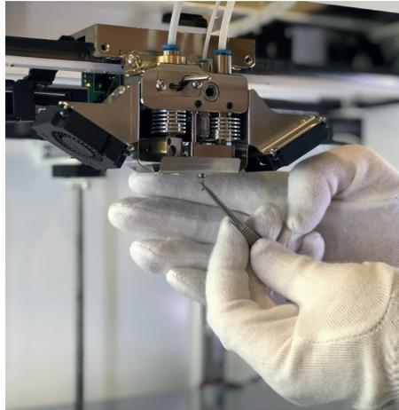
3. Clean the contact surface of the composite nozzle by brass wire brush from the set of cleaning tools (see point 2. from “COMPOSITE EXTRUDER CHANNEL CLEANING”, p. 22)
